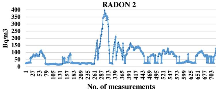
Fig. 6. Radon concentration between 7 June - 6 July 2018.
