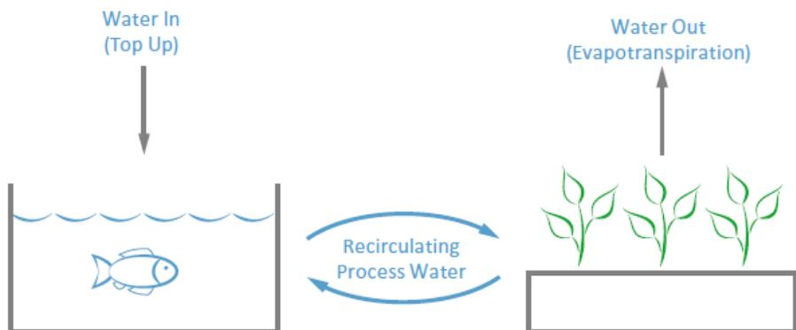
**Fig. 1.** Scheme of the water flow in an aquaponic system (by Lennard & Goddek, 2019)
