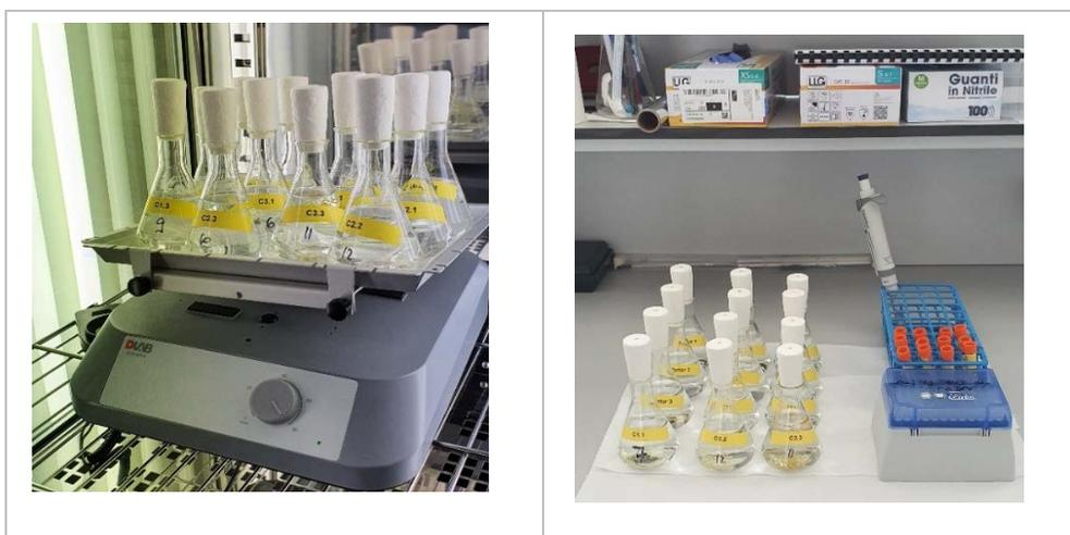
**Fig. 2.** Random positioning of the test containers on the 3D orbital shaker (left) and sampling (right)
